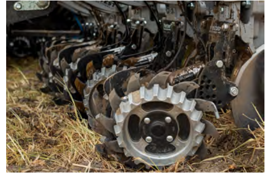
Figure 2. Yetter Row Cleaners with CleanSweep®
