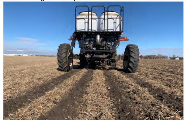
Figure 2. Strip-Till Banded Fertilizer
