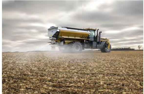
Figure 2. Strip-Till Banded Fertilizer with Montag® cart
