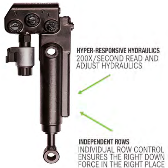
Figure 1. DeltaForce® Cylinder
