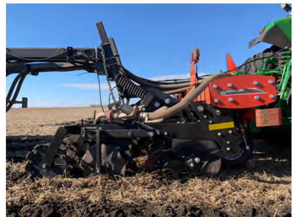
Figure 3. KUHN® Krause® strip-till unit
