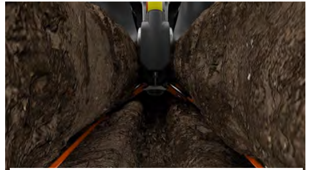
Figure 2. FurrowJet® In-Furrow Planter Attachment
