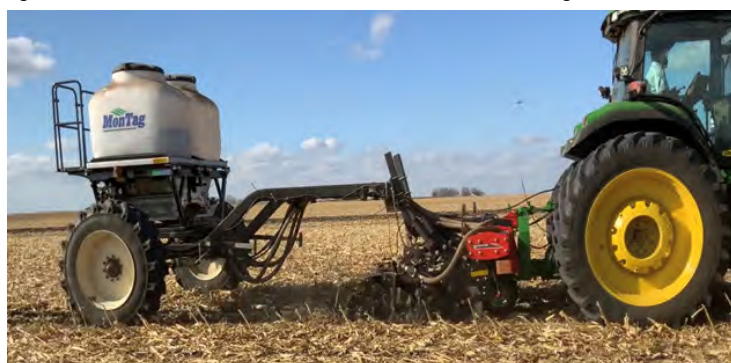
Figure 4. Kuhn® Krause® 1200 Gladiator® w/ Montag® Fertilizer Cart
