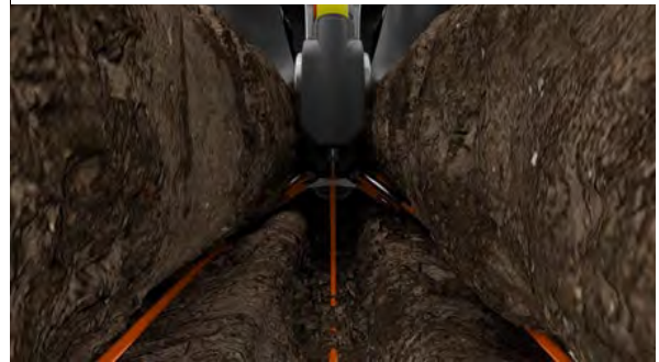
Figure 2: FurrowJet® Dual-Band Wings Fracturing Side-Walls
