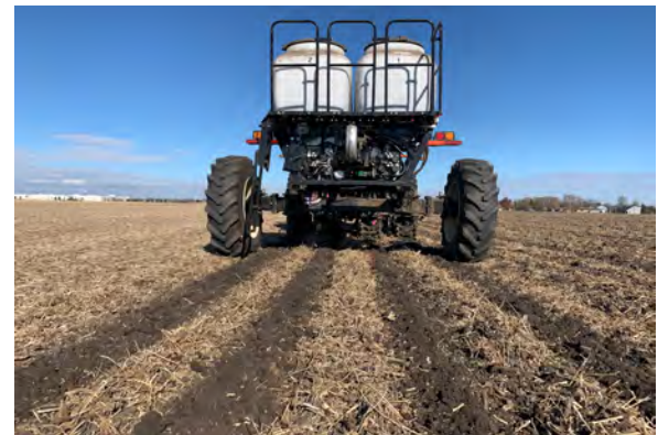
Figure 2. Strip-Till Banded Fertilizer
