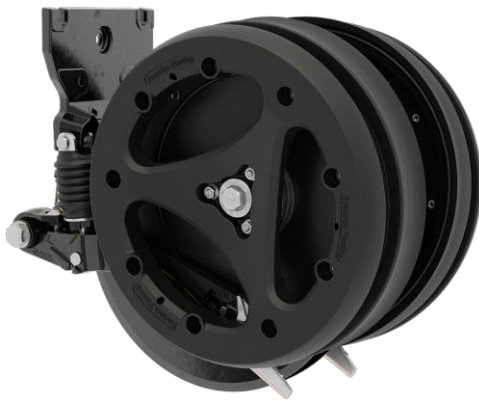
Figure 1. Conceal System Knife Design within Gauge Wheel
