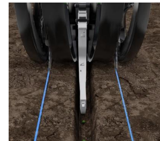
Figure 2. Conceal Dual Placement 3" from Seed Furrow, 1.5" in Depth
