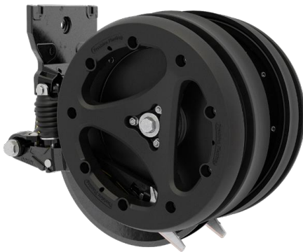
Figure 4. Conceal Knife Design within Gauge Wheel
