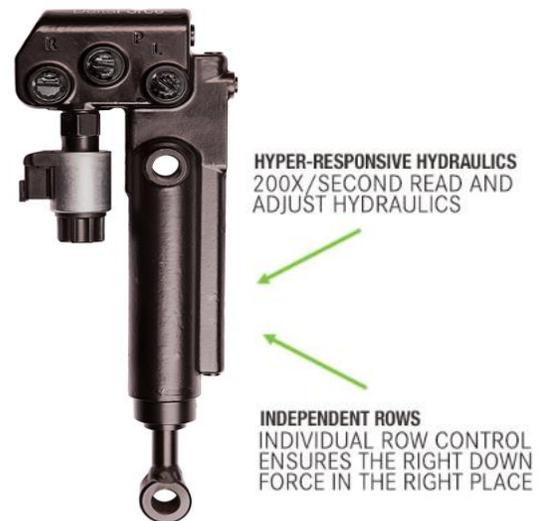
DeltaForce® system replaces the springs or air bags on your planter with hydraulic cylinders (Figure 1). It automatically increases or reduces weight with military precision, on each row individually. When one row encounters conditions different than another (wheel tracks, old roadbeds, clay knobs, headlands, etc.), each will adjust independently (Figure 2). Row by row, foot by foot, and seed by seed, you produce an environment that fosters uniform germination, optimum growth and maximum yield.
